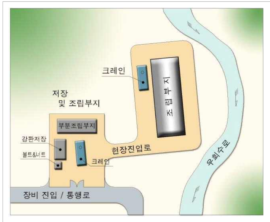
picture 4.1 basic steel plate construction
